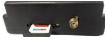
Place the SIM Tray in SLOT and Push the Tray
